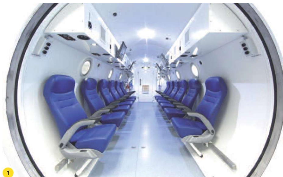
Image 1. Pressure cabine for the hyperbaric oxygen technology
